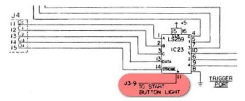
Your wiring harness may already have a wire coming from pin 9 (most likely yellow). If so, then install a wire from the molex connector on the other end to the control panel.
